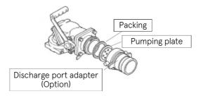
When you use the pump without a nozzle, put the pumping plate between the discharge port adaptor and the packing as shown in the figures above.
