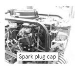
4. Measure the spark plug gap. If the gap is out of specification, replace the spark plug with the specified spark plug.
