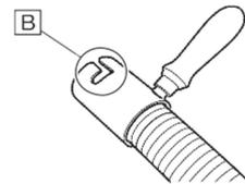
3. Turn the handle to fix exhaust pipe extension ②.
