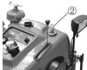
3. Operate the throttle dial to raise the pump pressure almost to 10 bar, and then check for water leaks from each part of the pump and the cooling water piping.
