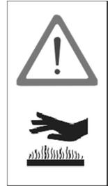
Always wear fireproof protective gloves when you handle the muffler exhaust pipe extension.
