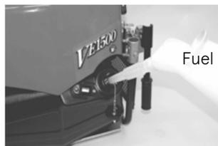
**Air vent is installed on the fuel filler cap. Close the cap tightly after refilling.**
