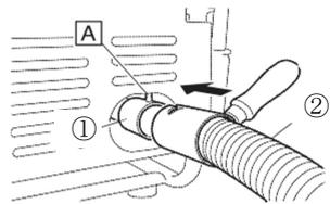
2. Fit notch [B] of exhaust pipe extension ② to boss [A] of muffler exhaust pipe ①.
