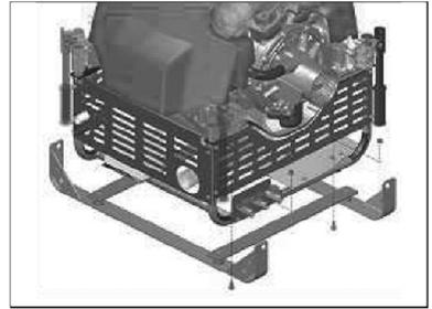
The TRANSPORTING DEVICE (TRANSPORT FRAME KIT) consists of the following parts.
