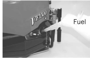
**Air vent is installed on the fuel filler cap. Close the cap tightly after refilling.**
